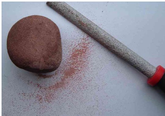
Figure 9a: sandstone scraped with a file
